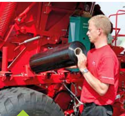
Fourteen film rolls: two on the ring and twelve underneath the guards.
